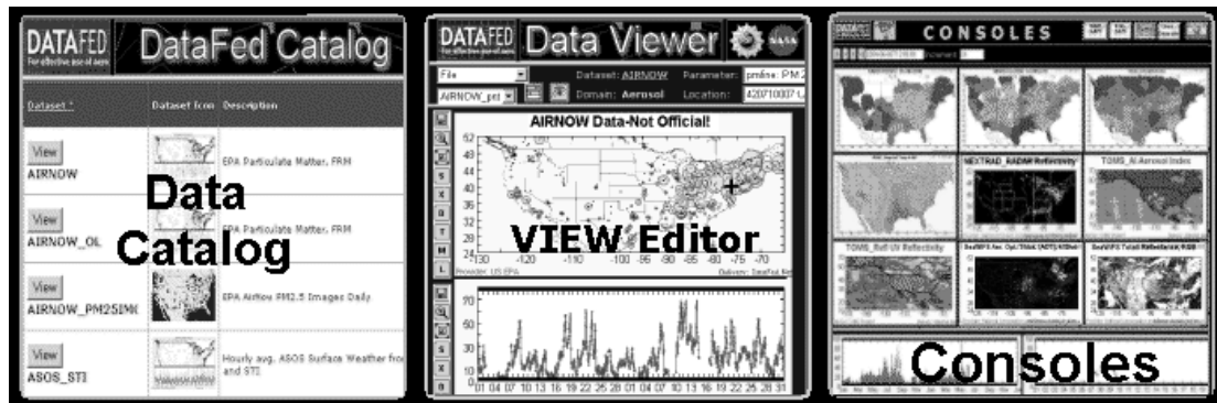
Fig 2. Main software programs of DataFed-FASTNET: Catalog for finding and selecting data, Viewer for exploration, and an array of Consoles for data analysis and presentation.
